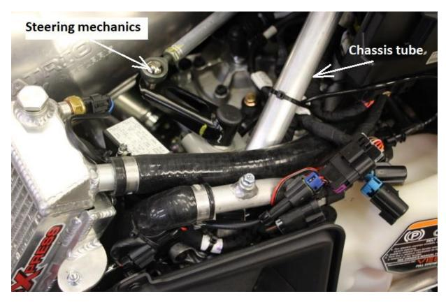
On the Polaris Khaos model, place the radiator hoses on the left side of the chassis tube like the picture.
