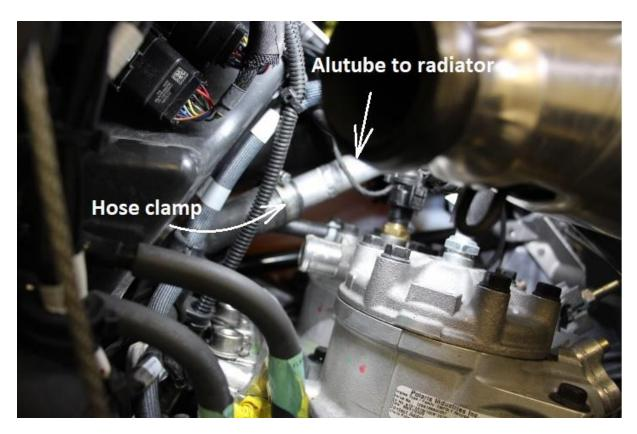
Install the aluminium tube like the pictures.
