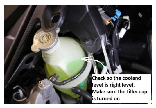
Before you fill up antifreeze in the new radiator, check the coolant level. The filler cap must be closed when filling the radiator.
