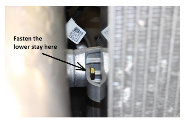
Install the radiator/fan on the sled. Use the same bolt as before.
