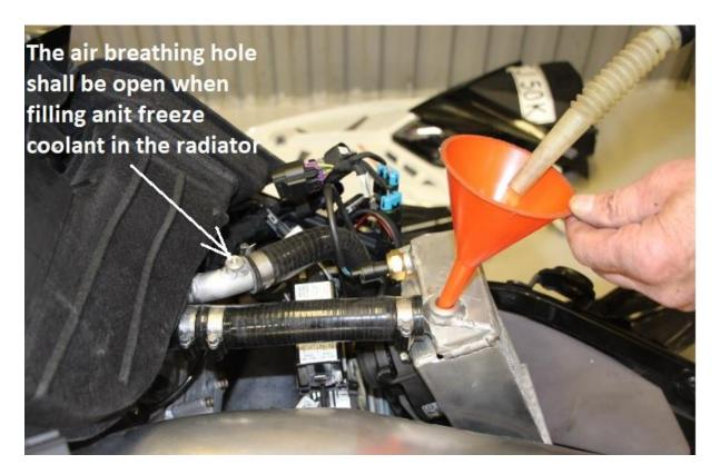
Fill up the radiator with antifreeze coolant until it come comes up in the air breath hole on the aluminium water tube.
