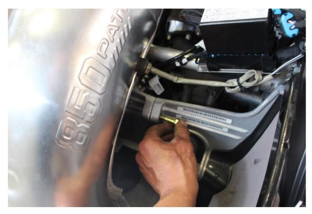
The lower stay for the water radiator will be fastened at this bolt.
