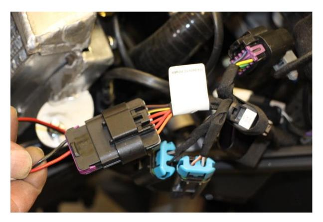
Plug in the fan connector to diagnostic power connector on the sled. (You will find this connector very close to the radiator)
