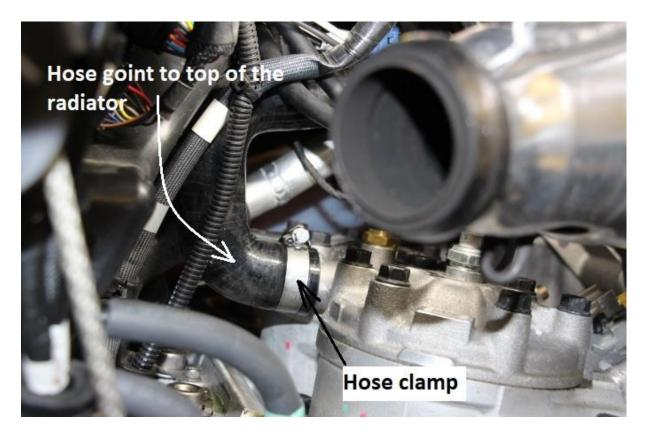
Install the hose between the cylinder head and the radiator
