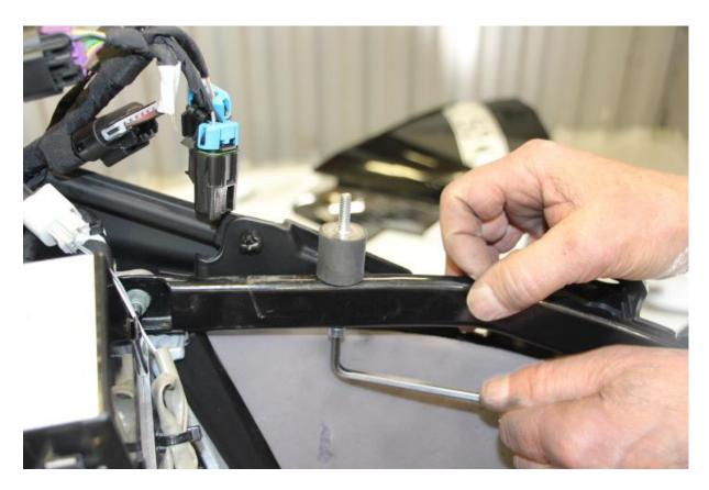
Install a rubber mount in this hole. Use an M6x35 bolt.
