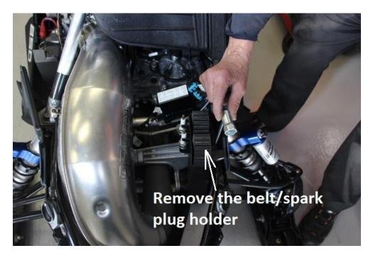
To make space for the cooler kit you have to remove the holder for the spare spark plugs and the spare belt.
