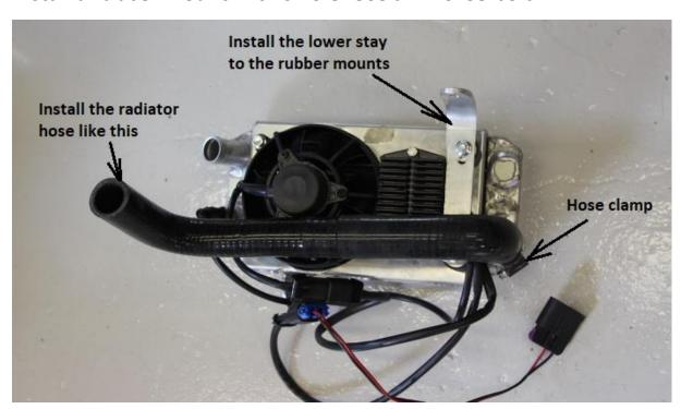
Install the lower radiator hose and the lower cooler stay like the picture.
