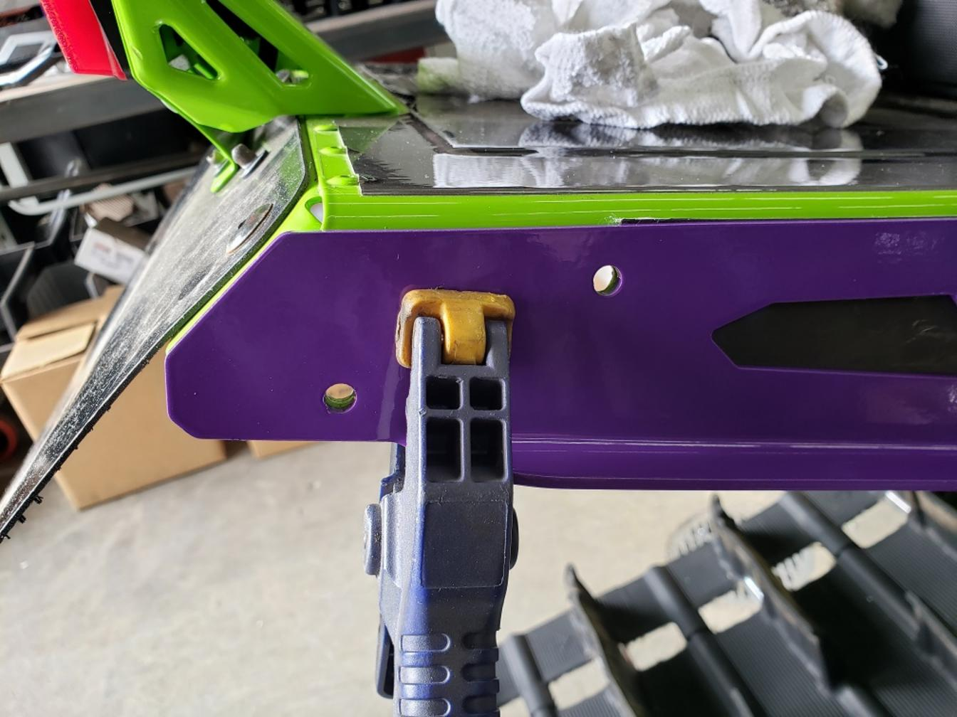
All circled rivets are SHORT RIVETS. Use a rivet washer on the tunnel side as well. Install all of these before proceeding to front section of bumper.
